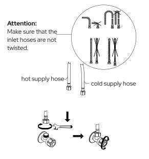
Then, Install the spray hose to the outlet hose. The outlet will connect with a simple push.
